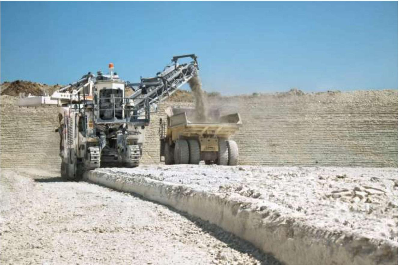
Figure A-1. A Wirtgen 4200SM Surface Miner.
