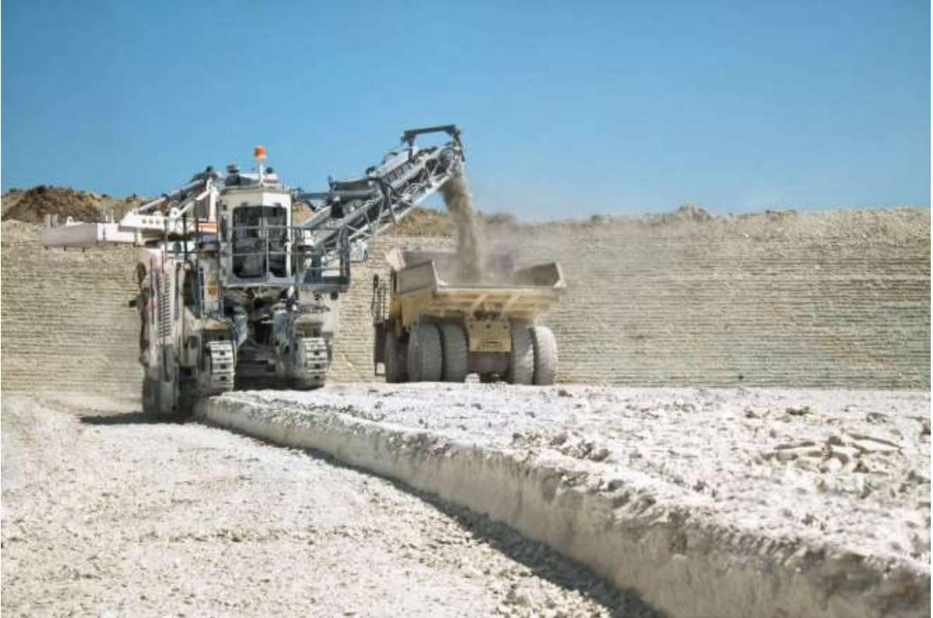
Figure B-4. A Wirtgen 4200SM Surface Miner.
