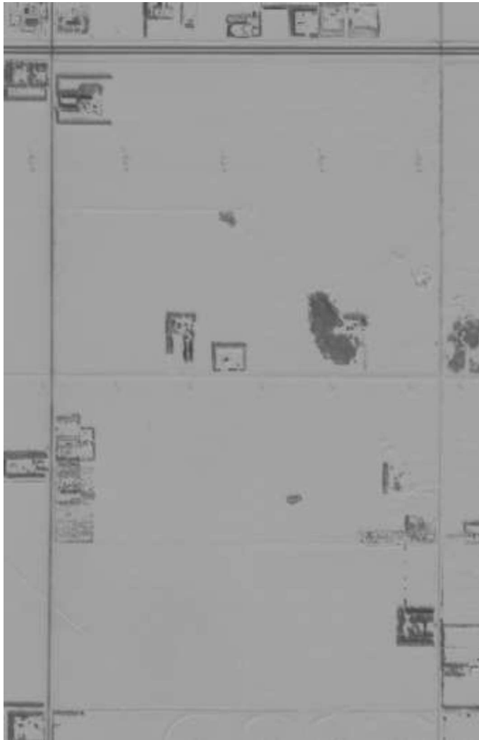
Figure 1-3. Prevalence of agriculture is reflected in unsupervised classification mapping of grey-toned “spectral signature” for cropland in recent satellite image. Darker polygons are shelterbelts, woodlots, houses, machine sheds, etc. Source: Google Earth, MLI3 Inc.
