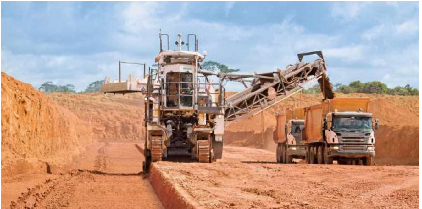
Figure B-6. A Wirtgen 2500SM Surface Miner.
